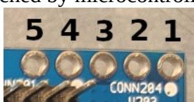
The supported steering wheel interface is the variable resistance to ground type, in which each button on the steering wheel will connect to ground through a distinct resistance. Together with the R20x resistor pulling the line up to 3.3v, each button will yield a different voltage in the range of 0-3.3v. The microcontroller is programmed to recognize the distinct voltages and issue USB-HCI commands to the SBC based on the button states.
