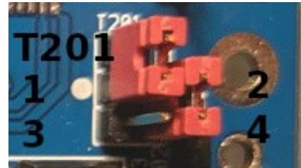
T201 is connected to the output of the same switch as CONN204-2.
