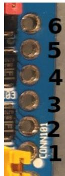
Note that it is not necessary to attach both ground pins. Additional ground connections are provided for convenience.
